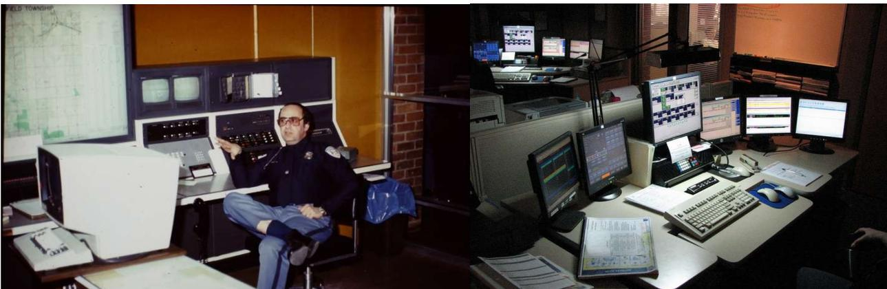
Above, the only thing these dispatch centers have in common is that they both belong to the Bloomfield Township Police Department. The dispatch center of the 70's and 80's (left) were loaded with huge cathode ray tubes (CRT's), and consoles with dozens of buttons and switches. The modern dispatch center (right) now integrates radio communications and telephone operations, all controlled with flat screen monitors and a computer mouse.
