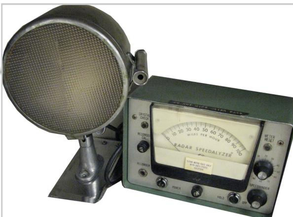
**Left,** There was a time when this radar unit was state of the art speed measurement equipment! The large antenna to the left was hooked to a patrol car's passenger window. Everyday, the unit had to be calibrated before patrol using the tuning forks (below).
