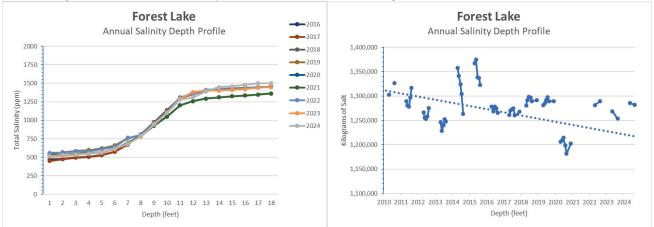
The first graph shows the average annual salinity at 3-foot depth intervals. This graph shows the salinity increases with depth and ranges from about 500 parts per million at the surface to about 1,500 parts per million in the deepest portion of the lake. This year, there wasn't a stark increase in the salinity in the deeper water, compared to previous years.
